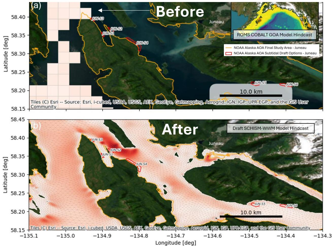
*Top: Existing current speed data (intended for regional-scale dynamics). Bottom: Data being generated by Kelson Marine in the present project. Close-up of Juneau, AK with NOAA Alaska draft AOAs.*
